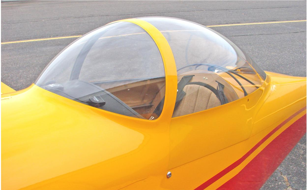
The scratch-built windscreen bow and canopy frame are welded 4130 steel tubing and the canopy skirt is fiberglass.
