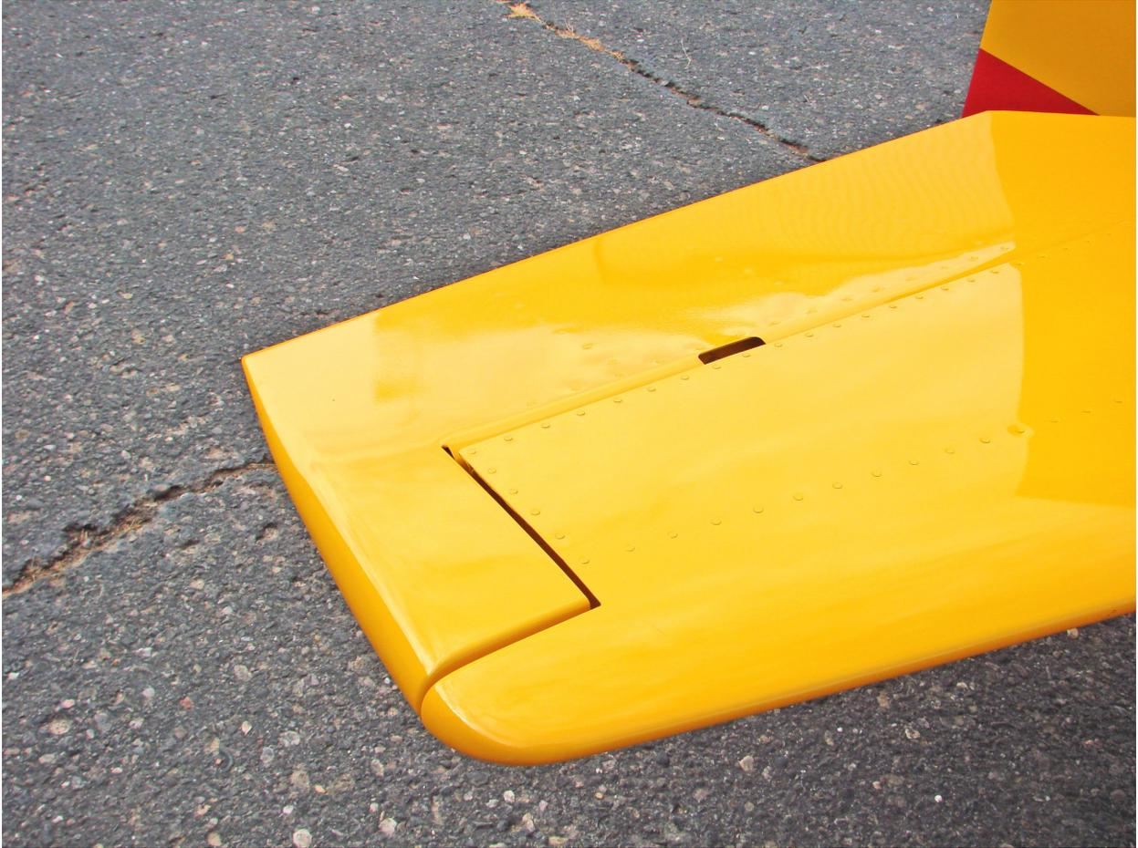
**Counter-balanced elevators (original design):**
