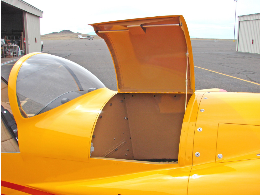
The door opens to a 14-inch deep, 1.75 cubic foot storage compartment with a 25-pound capacity.
