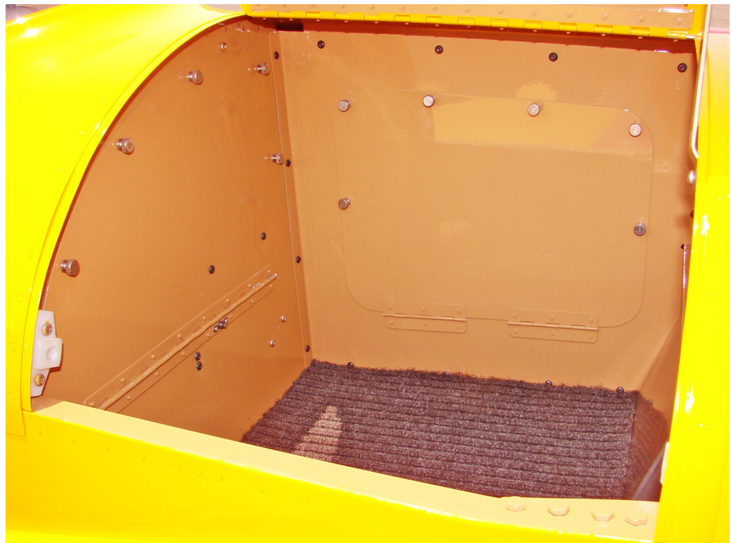
The door opens to a 14-inch deep, 1.75 cubic foot storage compartment with a 25-pound capacity.
