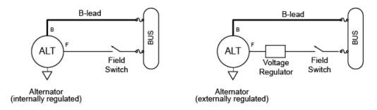
**B-lead**. The B-lead is the big wire (typically a 6 or 8 gauge wire) that runs from the alternator to the bus. It carries the power generated by the alternator to the bus, which then distributes it to the individual devices and to the battery. An electrical bus (alternatively spelled "buss") is a common electrical connection between multiple electrical devices. It can be a solid piece of copper or wires connected together.
