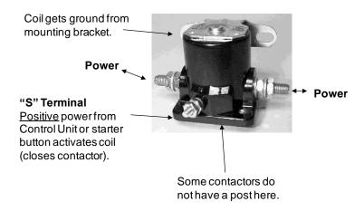
The starter contactor and master contactor are designed to be activated in different ways for safety reasons.
