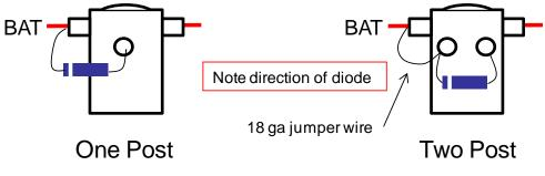
Battery Contactor Diode Installation
