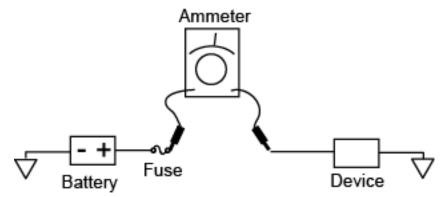
Connect the ammeter in series between the battery and the load.
