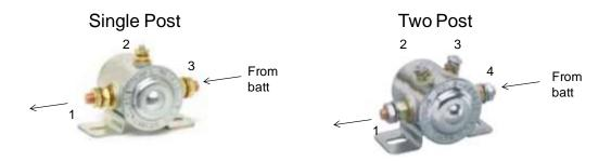
The starter contactor (aka starter relay) is an intermittent duty relay meaning it is designed to be turned on only for short periods of time. This contactor draws about 4A at 14v. You'll notice from the diagram below that the contactor coil is grounded via the bracket on the back of the contactor. Therefore, the starter coil is energized when +12v is applied to the small post (coil).
