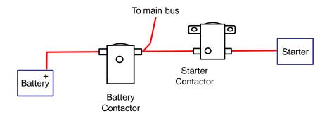
There are two types of contactors generally used in experimental aircraft. One is a continuous duty contactor (usually on) and the other is an intermittent duty contactor (only on for a few seconds at a time). Vertical Power provides an in-depth look at contactors here <u>http://verticalpower.com/docs/Contactor\_Wiring.pdf</u>
