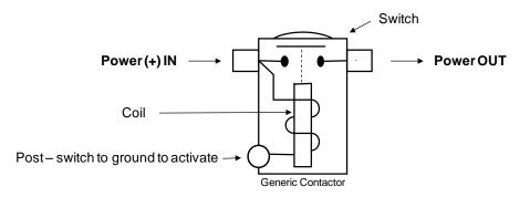
The master contactor is used to isolate the battery from the rest of the aircraft. Shutting it off (via the master switch) generally removes power from the aircraft and cockpit in case of an emergency.
