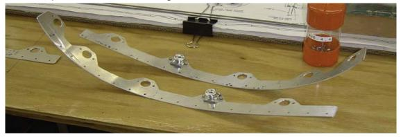
**INSTALLING FASTENERS AND GROMMETS:** Next, the center pilot holes in the cowling can be enlarged to accommodate the fastener grommets (15/32"). Use a UniBit (step drill) for this to make sure you get nice round holes. With the holes enlarged the grommets can be installed and the grommet retaining rings can be put on the back side
