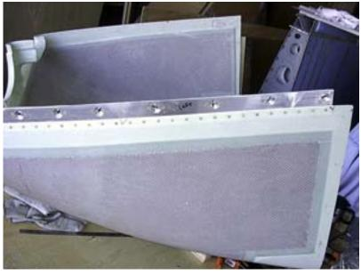
The support strips along the sides need at least 1-1/8" (preferably 1-1/2") width from the lower cowl edge (step) to the upper edge of the strip. This same dimension is required for the firewall support strips.
