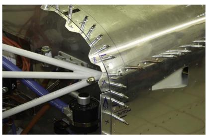
Also note that you will want to do some scalloping of the mounting strip between the receptacles that go around the top of the firewall. This is so the tabs can be slightly bent up or down to fit the contour of the cowl and fuselage.
