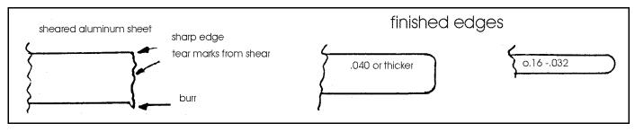
small cracks is that they soon become large cracks, one piece of aluminum becomes two pieces, etc. Obviously, we do not want this happening in our airframe, particularly when separated from solid earth by a lot of very thin air.
